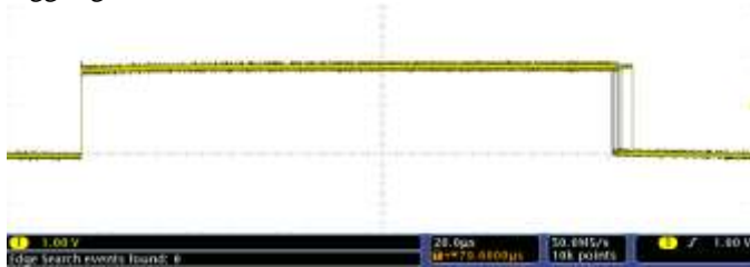
Figure 4. Scope output of GPIO toggling in the standart Linux
