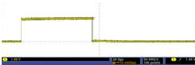
Figure 5. Scope output of GPIO toggling in Multi-scheduling enabled Linux
