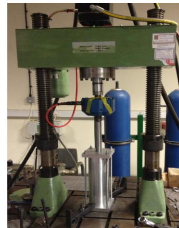
Figure 3: Set-up test rig on Servo Test System.
