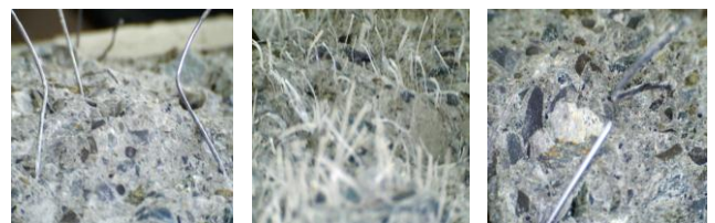
Figure 9. Distribution of steel and polypropylene fiber in the concrete.
