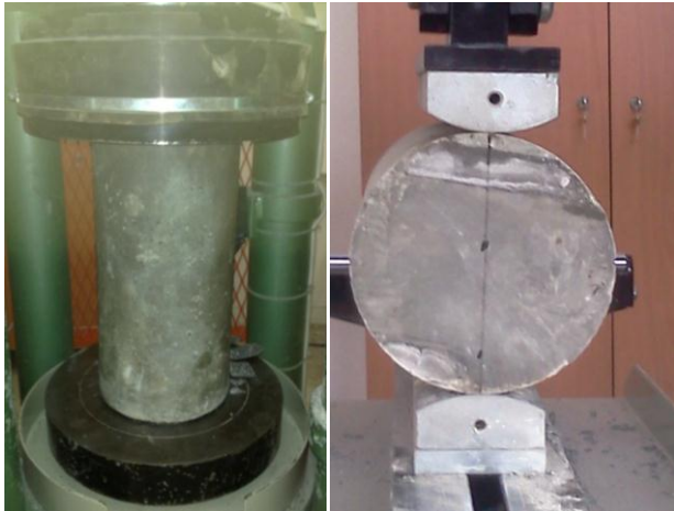
Figure 4. Compressive strength and tensile strength on split experiment.
