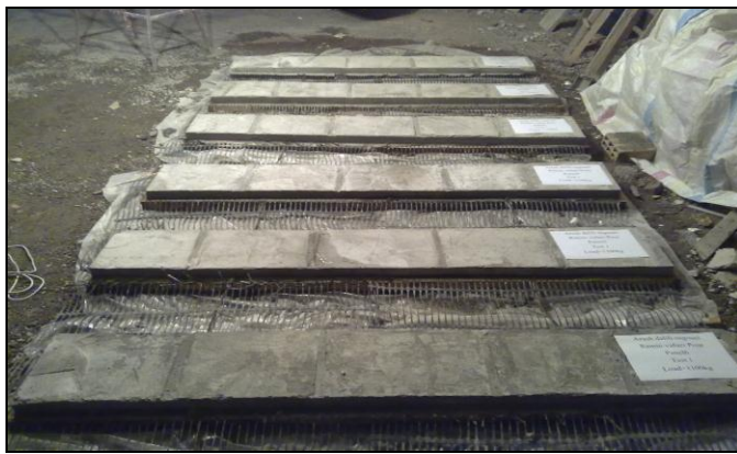
Figure 1. Concrete mats are made in the laboratory
