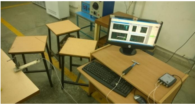
Figure 4: Impulse hammer experimental setup
