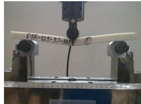
Figure 3. Three-Point bending testing of 125kg/m 3 12:1 specimen on Instron machine
