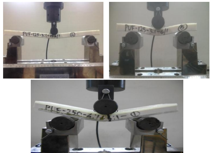
Figure 3: Specimens under three point bending test of 15.4:1, 12:1 & 6:1 span to depth ratio
