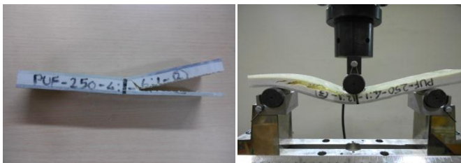
Fig 11: Skin and Core localized damage in 3:1 & 4:1 skin-core ratio of 250 kg/m 3 density foam specimen
