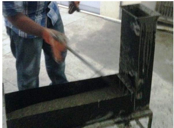
Fig.2. L-Box Test (Passing Ability)
