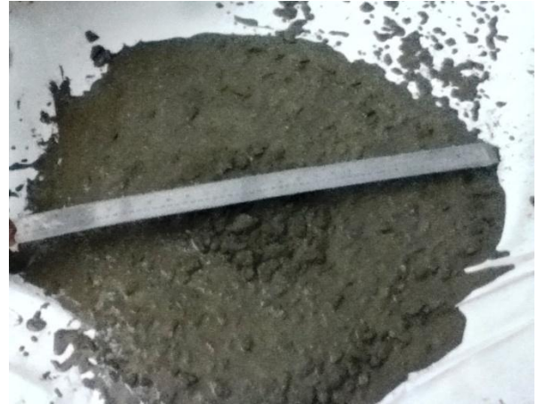
Fig.1: Slump test (Flow ability)
