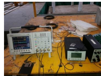
Figure3. Instrumentation for Pitch catch configuration method
