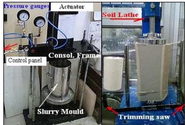
Fig. 2. Consolidation setup on the laboratory floor
