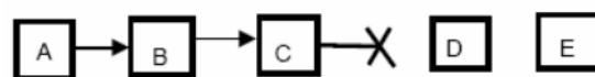
Fig.2 Node C is unable to forward a packet from A to E over the next node D
