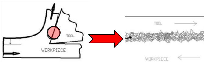
Figure 12. Rolling elements in the tool-chip interface [16]
