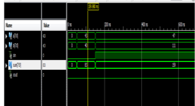
Fig 3. Stimulation Result of 8 bit ripple carry adder
