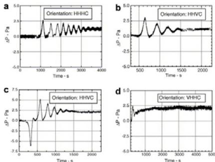
Fig. 13. Flow initiation for different orientations. (a) Flow initiation in the anticlockwise direction at 102 W, (b) flow initiation in the anticlockwise direction at 128 W, (c) auto flow reversal in case of initiation in the clockwise direction at 257 W and (d) flow initiation in the anticlockwise direction at 530 W.
