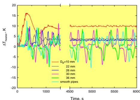
Fig. 19. Comparison between tests with smooth pipes and pipes with orifices (P=500 W).
