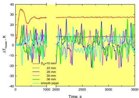
Fig. 20. Comparison between tests with smooth pipes and pipes with orifices (P=2500 W).
