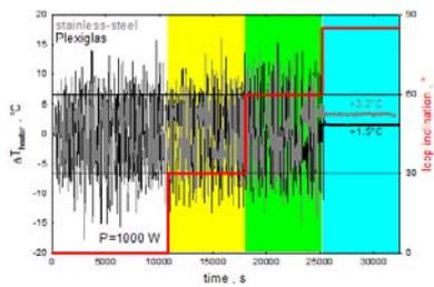
Fig. 10. Temperature difference across the heater  $\Delta T_{\text{heater}}$  vs. time for two connecting materials, colours background correspond to different loop inclinations. ( $P=1000 \text{ W}$ ,  $\text{FC43}$ ).
