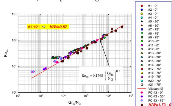
Fig. 28. Comparison between experimental data and Vijayan’s correlation
