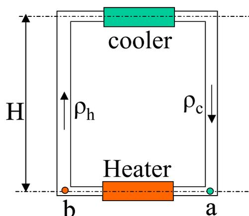
Fig. 1. Single-phase Natural Circulation Loop (NCL)
