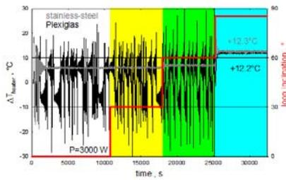
Fig. 8. Temperature difference across the heater  $\Delta T_{\text{heater}}$  vs. time for two connecting materials, colours background correspond to different loop inclinations. ( $P=3000 \text{ W}$ ,  $\text{H}_2\text{O}$ ).
