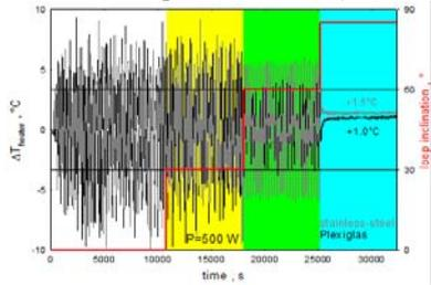
Fig. 9. Temperature difference across the heater  $\Delta T_{\text{heater}}$  vs. time for two connecting materials, colours background correspond to different loop inclinations. ( $P=500 \text{ W}$ ,  $\text{FC43}$ ).
