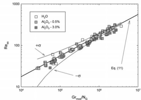
Fig. 29. Comparison between experimental data and Vijayan’s correlation.
