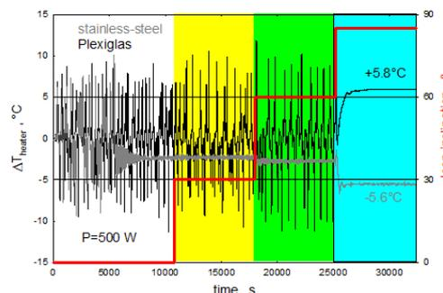
Fig. 7. Temperature difference across the heater  $\Delta T_{heater}$  vs. time for two connecting materials, colours background correspond to different loop inclinations. (P=500 W, H<sub>2</sub>O).
