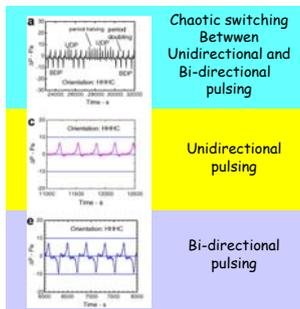
Fig. 14. Various unstable oscillatory modes observed with change in operating conditions for the HHC orientation.
