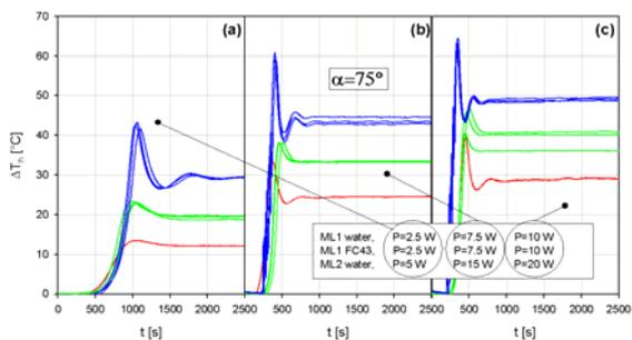
Fig. 27. Transient behaviours of  $\Delta T_h$  for  $\alpha=75^\circ$ .
