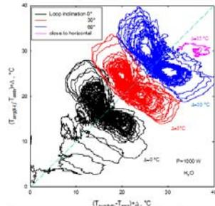
Fig. 11 Trajectories of average temperature difference bottom left vs. average temperature difference bottom right ( $P=1000 \text{ W}$ ,  $\text{H}_2\text{O}$ ).
