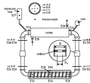
Fig. 18. Sketch of the rectangular loop. The localized pressure drops (orifices of different diameter) are placed in the middle of vertical legs.
