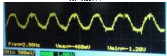
Fig. 1c: Dynamic loading sine wave output shown on Oscilloscope for -1.2800V
