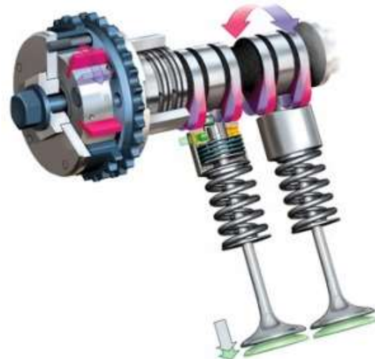
CAM operation according to variable valve timing
