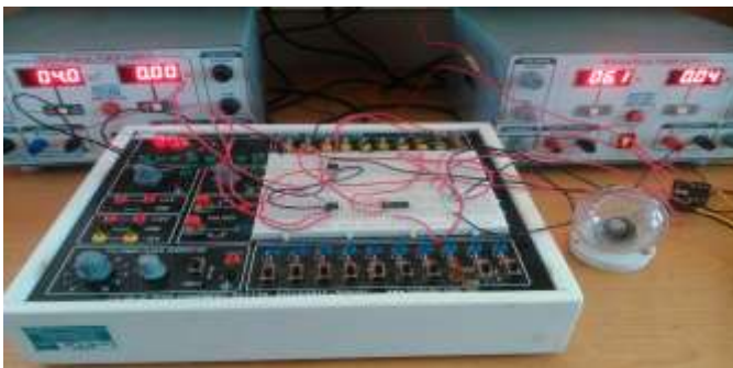
Figure 9. Voltage based electronic fuse circuit operation above the specified voltage range. (Off Condition)
