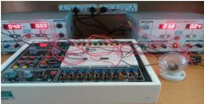
Figure 8. Voltage based electronic fuse circuit operation below the specified voltage range. (Off Condition)
