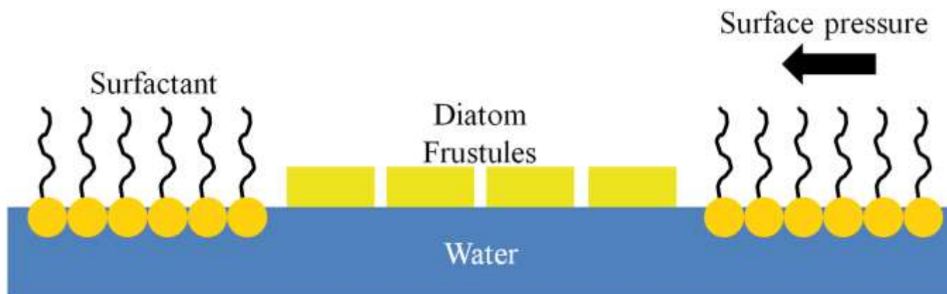
Figure 4. Schematic of the self-assembly of diatom frustules in a Langmuir trough.
