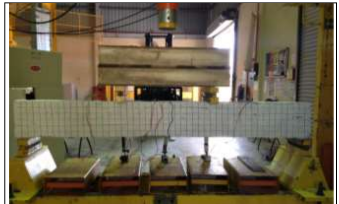
Figure 4. Flexural capacity test setup
