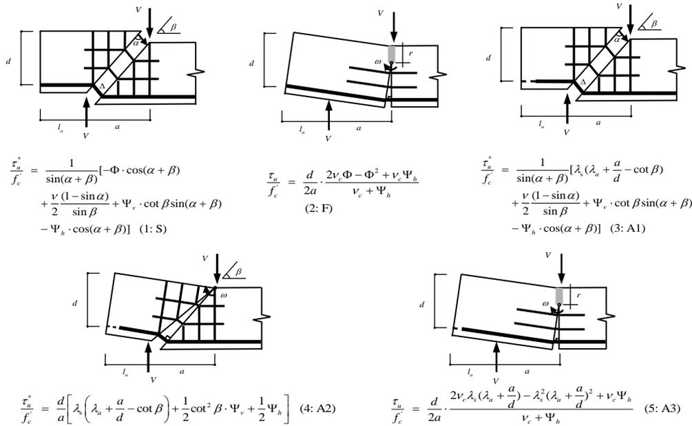
Figure 1. Failure mechanisms and shear strength equations. [1]
