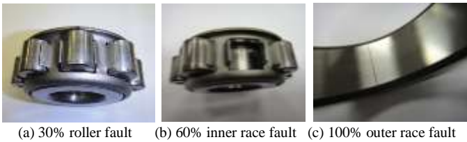
Figure 6. Photo of fault bearing
