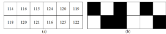
Fig. 5. (a) Cover image of size 2 \times 6 . (b) The 3^{\text{rd}} bit plane of the cover image given in (a).
