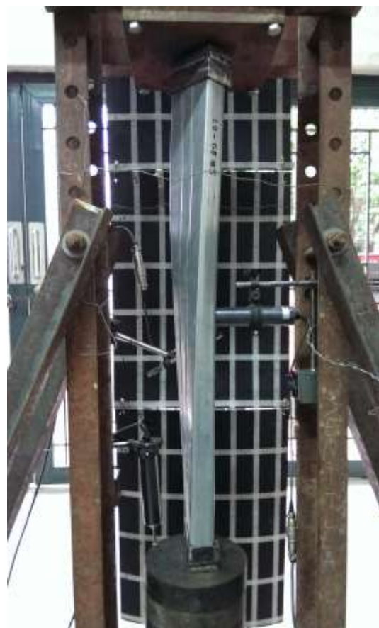
Figure 2. Concentric compression loading of specimen showing buckling failure
