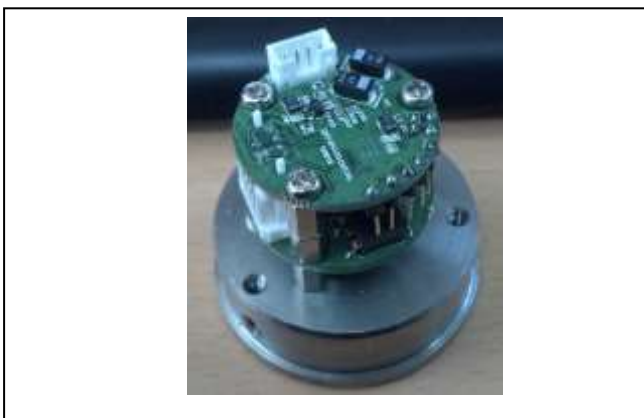
Figure 2. Interior structure of inclinometer
