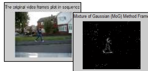
Fig.4 Background Subtraction using Mixture of Gaussian
