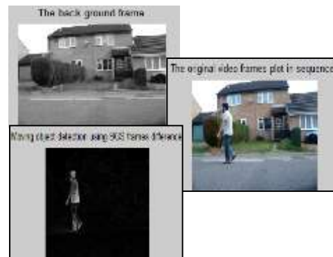
Fig.1 Background Subtraction using Frame Difference
