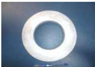
Figure 1. FGMMC Cast Ring
