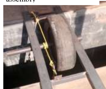
Fig. 3b - The final prototype of the single roller unit
