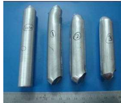
Fig. 3 Photograph of ECAE samples before and after extrusion
