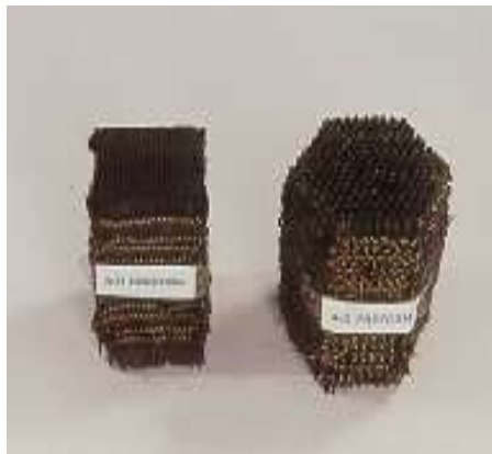
Fig: 7 3D, 4D woven preforms
