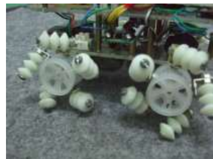
Figure 4. Mecanum Wheels using Abacus Beads
