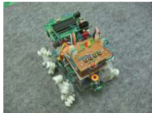
Figure 3. Multi-Movement Mobile Robot using Mecanum Wheels
