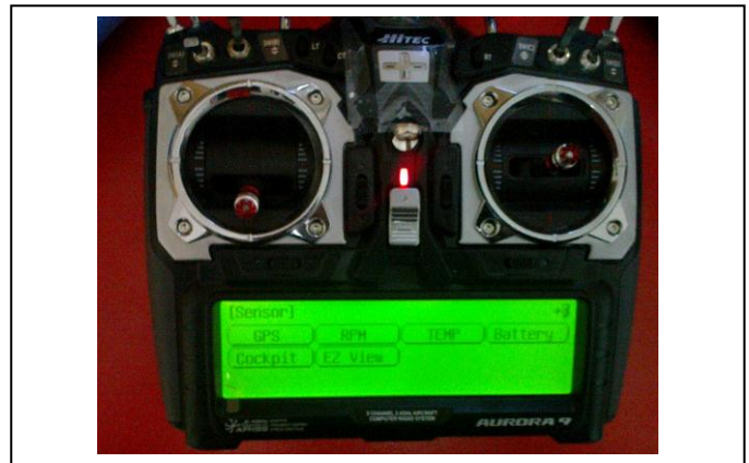
Figure 3. The the remote control device's screen relating the sensors
