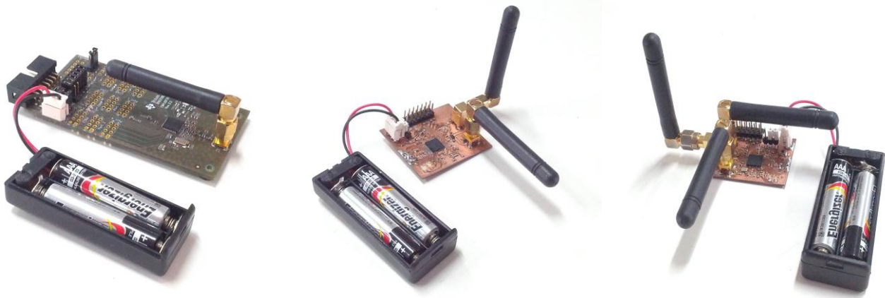
Figure 3. a) Regular sensor node b) Two-antenna node c) Three-antenna node
