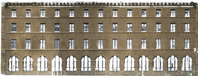
Figure 4. Visualization of the 95 dense point clouds generated by SURE.
