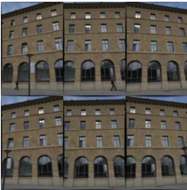
Figure 2. Images captured from proximate camera stations, at each station 3 images were collected with slight variances in viewing directions.
