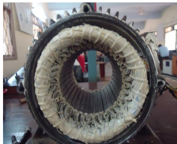
Figure 2 Nanocomposite filled enamel coated induction motor
