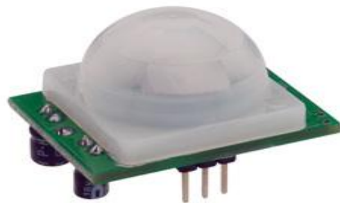
Figure 6 Passive Infra-Red Sensors (PIR)
