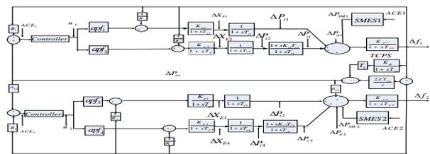
Fig. 4. Two areas reheat thermal power system model.
