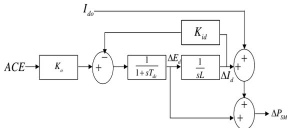
Fig. 2. Block diagram of SMES control scheme [3].
