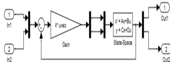
Figure1: LQR Simulink Model for CSTR Model
