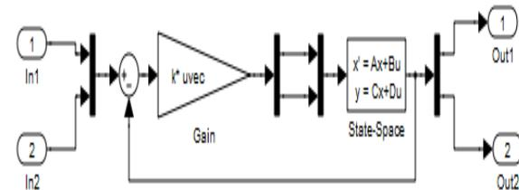
Figure1: LQR Simulink Model for CSTR Model
