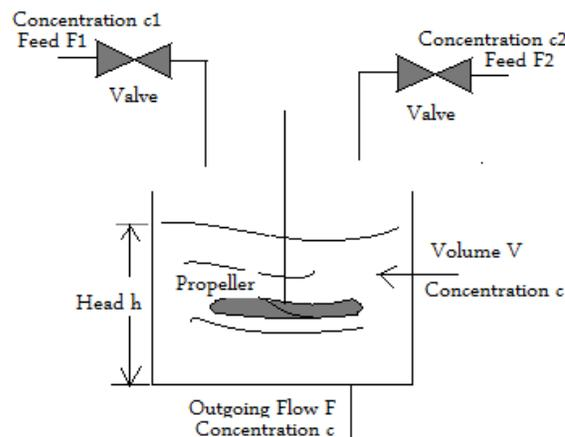
Figure 1: Schematic model of continuous stirred tank reactor
