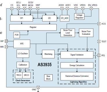
The external antenna is directly connected to the Analog Front-end (AFE), which amplifies and demodulates the received signal. The watchdog continuously monitors the output of the AFE and alerts the integrated lightning algorithm block in the event of an incoming signal. The lightning algorithm consists of hardwired logic.
