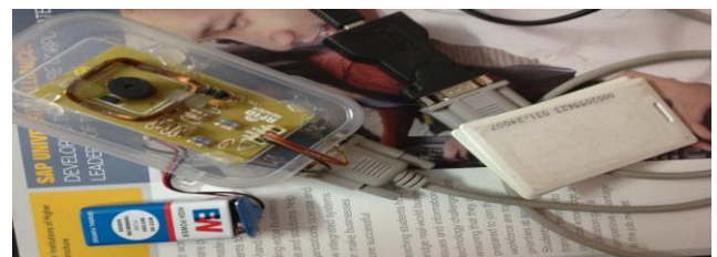
Fig. 8 RFID reader with RS 232 kit.
