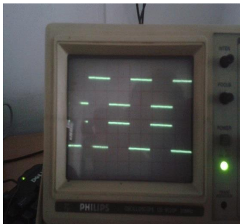
Multilevel PWM single phase experimental results at M_a \geq 0.5
