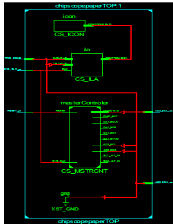
Figure 4. Internal view of Register Transfer Level (RTL) Synthesis result showing interconnection of “masterControler”, “icon”, “ila” modules within the top level entity “chipscopepaperTOP”.
