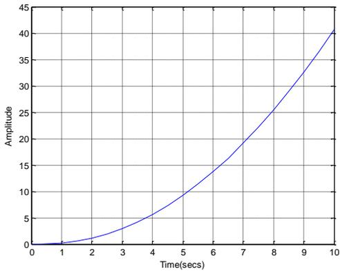
Fig.5. Step response of the plant without controller
