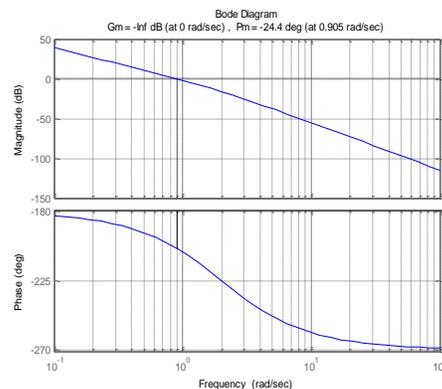
Fig.4. Bode plots of the system without controller
