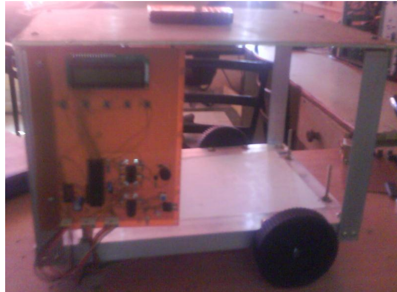
Figure 5. Line follower based Hospital Service Robot
