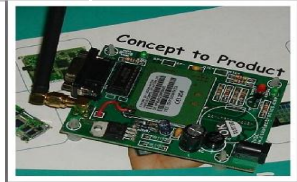
Fig.5 OPERATIONAL BOARD OF GSM MODULE ADDITIONAL ACCESSORIES
