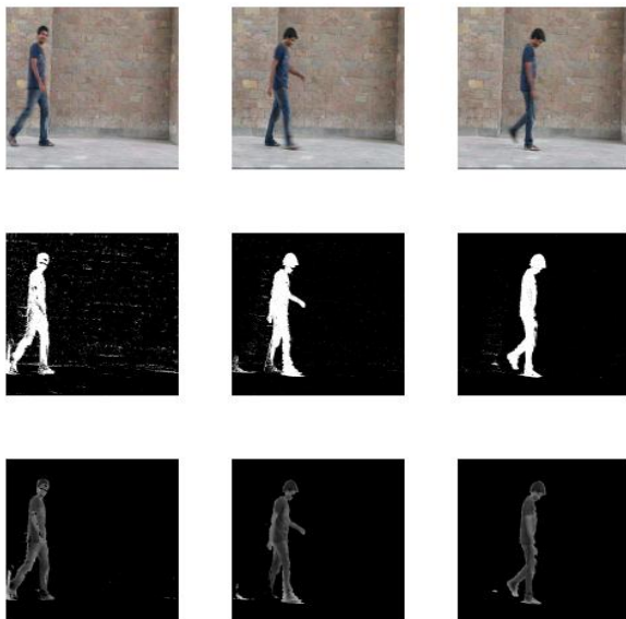
Figure 15: Background subtraction results of data set. The first row shows input video frames, second row shows background subtracted frames and third row shows the background subtraction results after median filtering.
