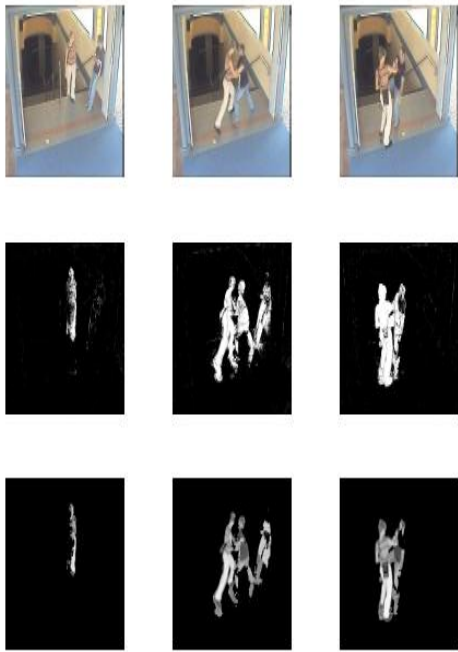
Fig. 4. Background subtraction results. The first row shows input video frames. Second row shows background subtracted frames. Third row shows the background subtraction result after median filter.
