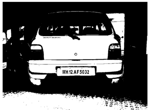
Fig.3 Output of Otsu’s algorithm
