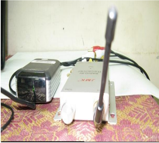
Fig. 8 Video receiver unit at control room
