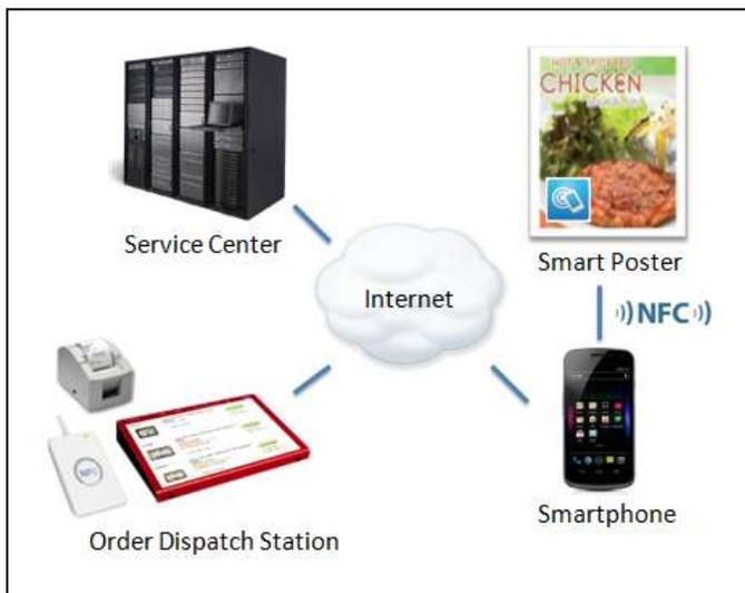
Figure 2. Solution Architecture
