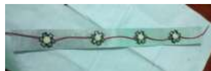
Fig 5: Back-side of the white LED panel showing series configuration.
